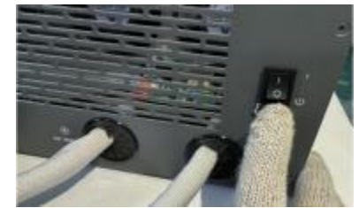
To complete the above steps, wait for one minute before starting the inverter switch
