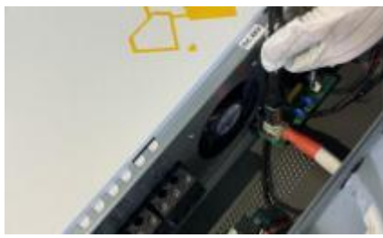
Connect the positive wire of the inverter
